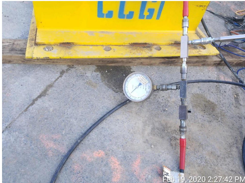
Micropile Load Test – South Abutment
