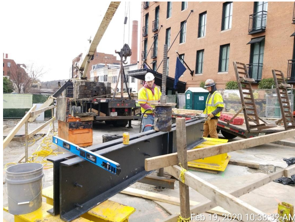
Micropile Load Test – South Abutment
