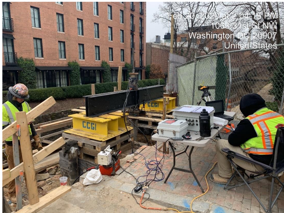
Micropile Load Test – North Abutment
