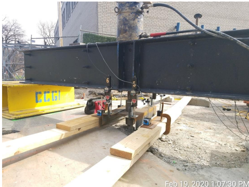
Micropile Load Test – South Abutment
